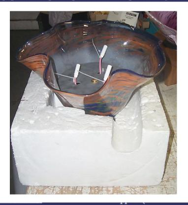
towels or newspapers crumpled up inside to keep the body stationary). In this position, one can see three female style quick-connects protruding through the three holes in the plexiglas circle. Next to each of these three holes, one can also see a nylon screw with a nylon cap nut penetrating through the plexiglas. First, remove each nylon cap nut from each nylon screw.
